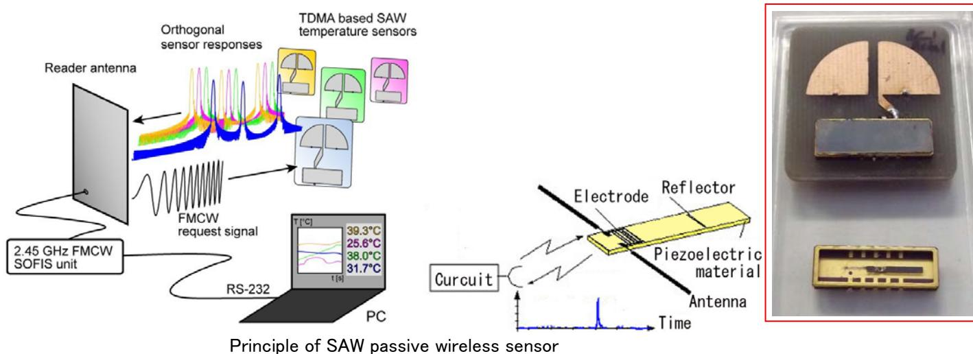
Reference : J. H. Kuypers, L. M. Reindl, S. Tanaka and M. Esashi, Maximum Accuracy Evaluation Scheme for Wireless SAW Delay Line Sensors, IEEE Transactions on Ultrasonics, Ferroelectrics, and Frequency Control, 55 (2008) pp.1640–1652
