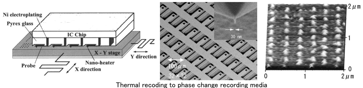
Reference : D.W.Lee, T.Ono, T.Abe and M.Esashi, Microprobe Array with Electrical Interconnection for Thermal Imaging and Data Storage, J. of Microelectromechanical Systems, 11 (2002) pp.215–219
