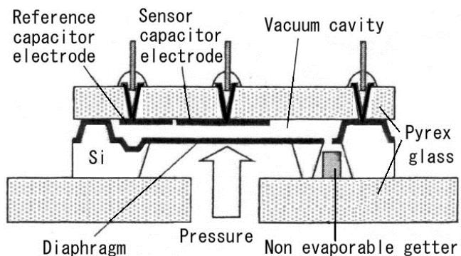
Reference : H. Miyashita, Y. Kitamura, Micromachined Capacitive Diaphragm Gauge, Anelva Technical Report, 11 (2005) pp.37-41 (in Japanese)
