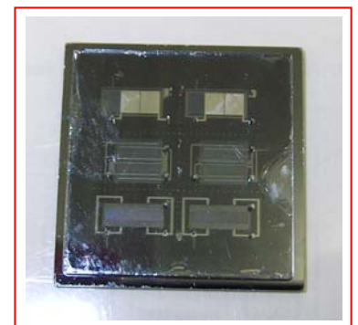
Capacitive accelerometer using deep RIE of SOI wafer with thick buried oxide (Tohoku Univ. – Daimler-Chrysler)
