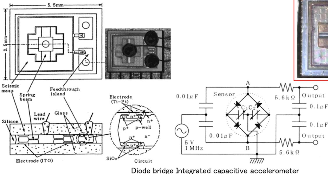
Diode bridge Integrated capacitive accelerometer
