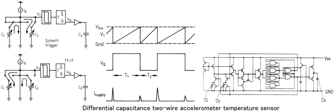
Differential capacitance two-wire accelerometer temperature sensor
