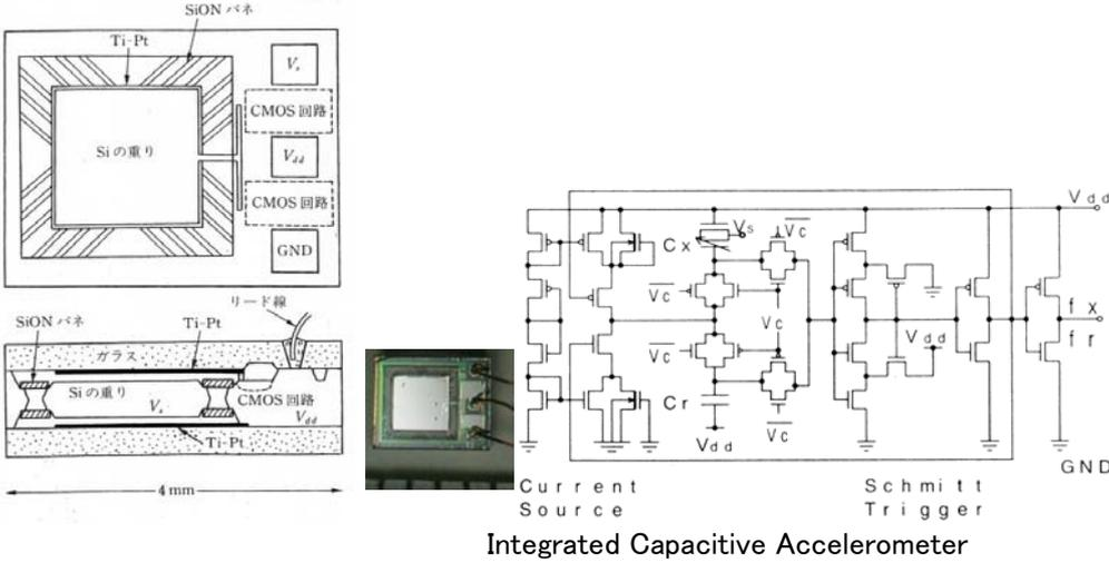
Integrated Capacitive Accelerometer
