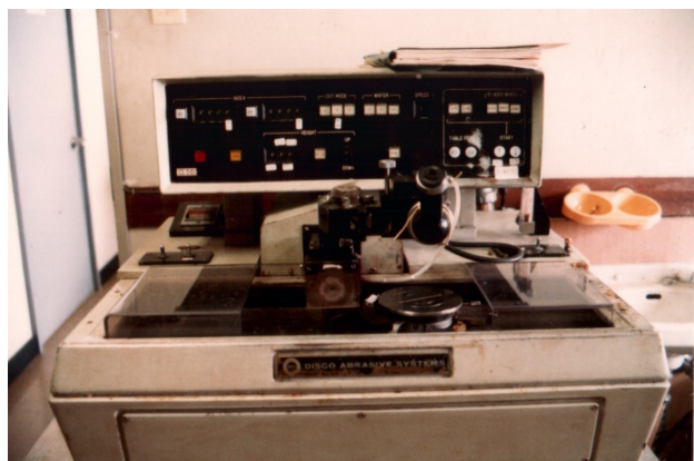
Dicing machine (chip separation from wafer)
