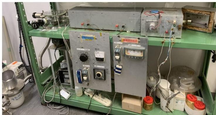
Parylene (Polyparaxylylene) deposition
