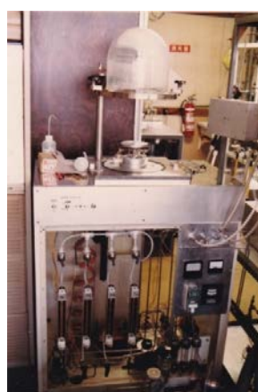
Low temperature SiO 2 CVD (exhibited)
