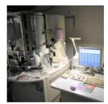
Scanning electron microscope (SEM)
