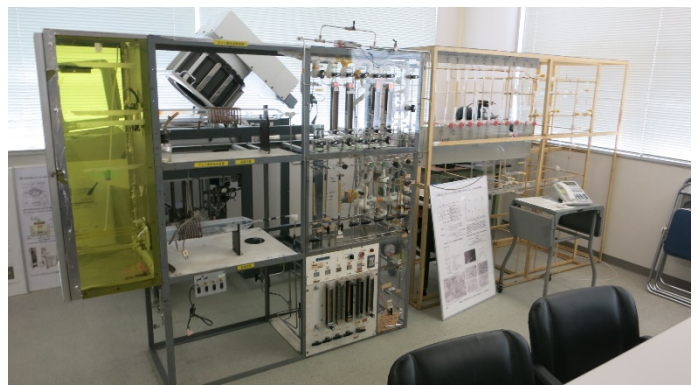
Glass pipe gas line for Si epitaxial growth system (right), atmospheric pressure CVD system (poly Si, Si 3 N 4 , SiO 2 ) (left)
