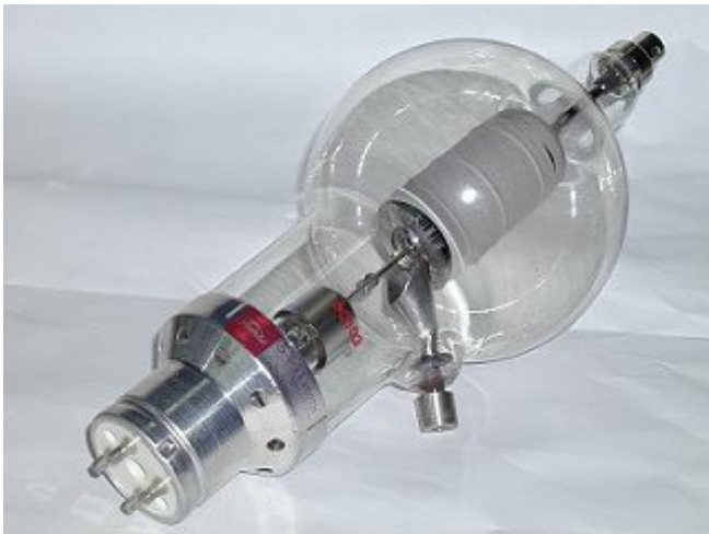
Triode for transmitter (5T31)
