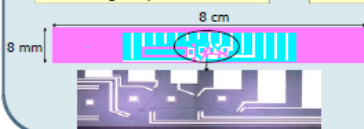
Sample for piezoresistive measurements with 4 differently orientated resistors
