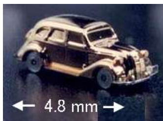
1/1000 size model of Toyota AA model (1936) (62 mg, 24 parts)
