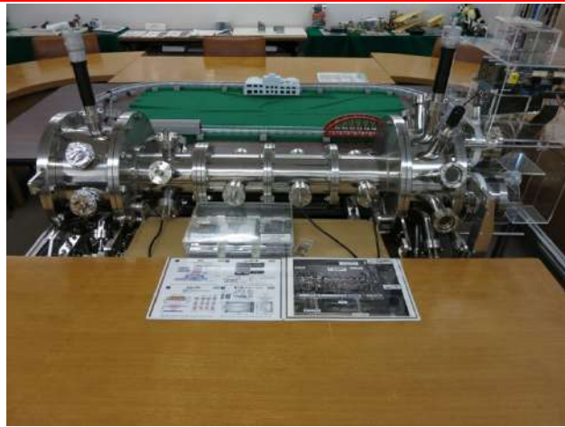
Massive parallel electron beam write using 100 \times 100 active matrix electron sources (right)
