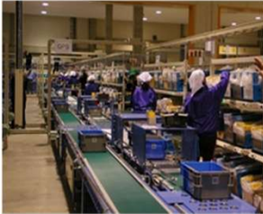
Piece picking at distribution centers, especially EC related ones
