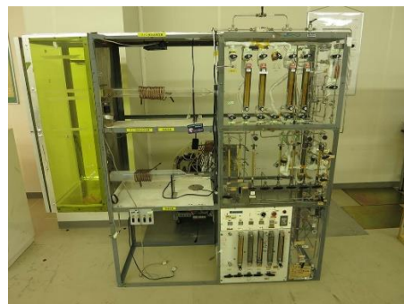
F. Atmospheric pressure CVD (poly Si, Si 3 N 4 , SiO 2 ) and RF power source for heating (backside)
