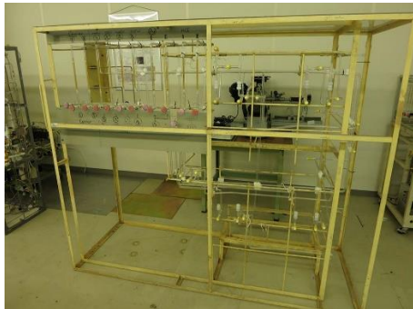
E. Glass pipe for Si vapor phase epitaxial growth and metal microscope (backside)
