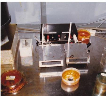
Spinner for resist coating and baking tool
