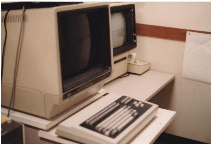
Graphic display connected to LSI11 (DEC) for LSI design
