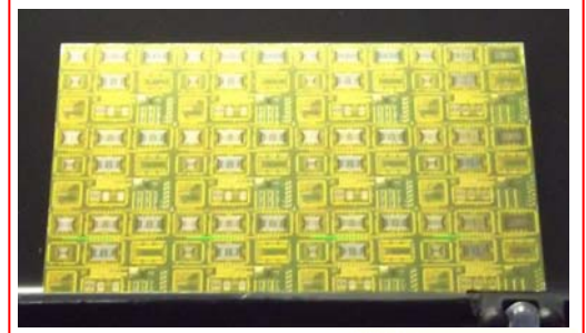
Exhibit #2: First poly-SiGe above-CMOS integrated gyroscope. The CMOS technology used is a standard 0.35 μm technology with 5 interconnect levels.
