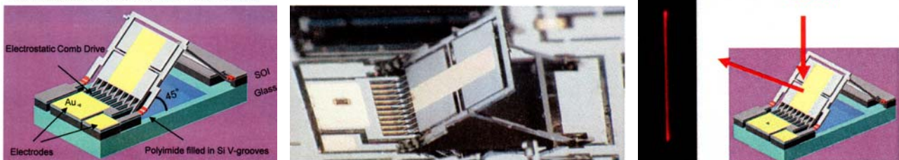
Electrostatic optical scanner for barcode reader (Tohoku Univ. - Optoelectronics)
