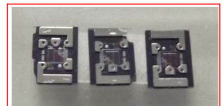
Tactile sensor network with polling type common 2-wire
