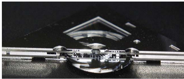
Si air-turbine with radial-inflow type journal bearing
