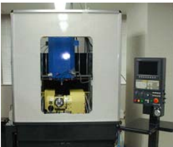
5 axis stage high speed spindle milling machine used for shaping turbine blade (Toshiba machine F-MACH)
