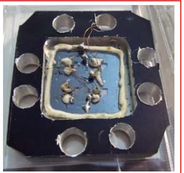
SiC diaphragm anti-corrosive vacuum sensor
