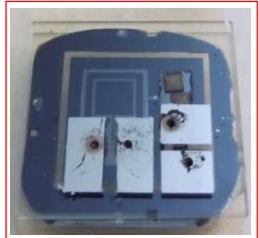
Vacuum encapsulation by anodic bonding with getter
