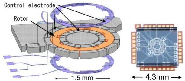
Yaw rate & acceleration sensor (Toyota motor Ltd.)
