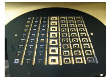
Three axis capacitive accelerations sensor achieved by a trainee
