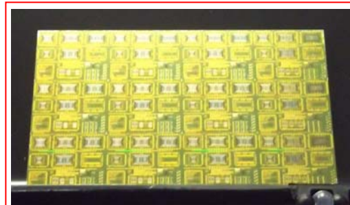
Exhibit #2: First poly-SiGe above-CMOS integrated gyroscope. The CMOS technology used is a standard 0.35 \mu\text{m} technology with 5 interconnect levels.
