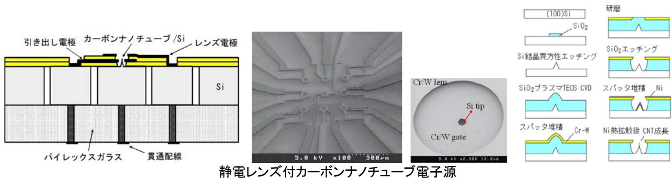
参考文献 : J.Ho, T.Ono, C.-H Tsai and M.Esashi, Photolithographic Fabrication of Gated Self-aligned Parallel Electron Beam Emitters with a Single-stranded Carbon Nanotube, Nanotechnology, 19 (2008) 365601(5pp)
