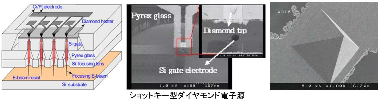
参考文献 : C.-H.Tsai, T.Ono and M.Esashi, Fabrication of Diamond Schottky Emitter Array by Using Electrophoresis Pre-treatment and Hot-filament Chemical Vapor Deposition, Diamond and Related Materials, 16 (2007) pp.1398-1402
