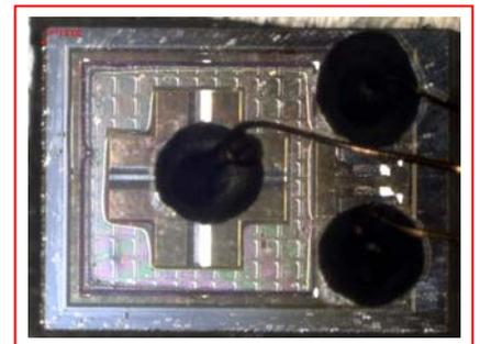
参考文献 : Y.Shoji, M.Yoshida, K.Minami and M.Esashi, Diode Integrated Capacitive Accelerometer with Reduced Structural Distortion, Transducers'95 (1995) pp.581-584
