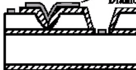
(6) Fe/Cr evaporation, lift-off or selective growth Diamond
