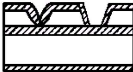
(3) Thermal oxidation (1.5 μm)
