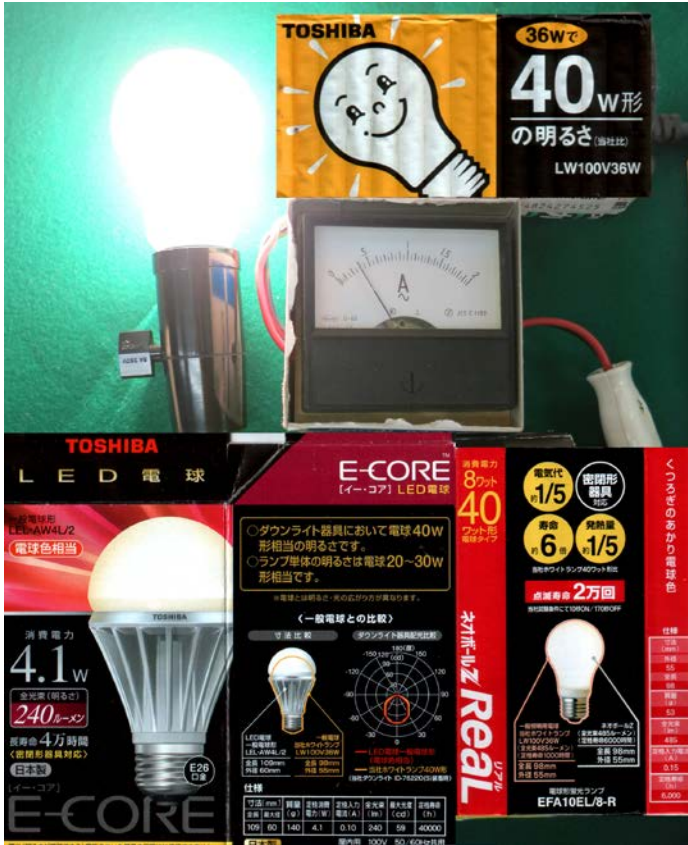
Current measurement of incandescent lamp, fluorescent lamp, and LED
