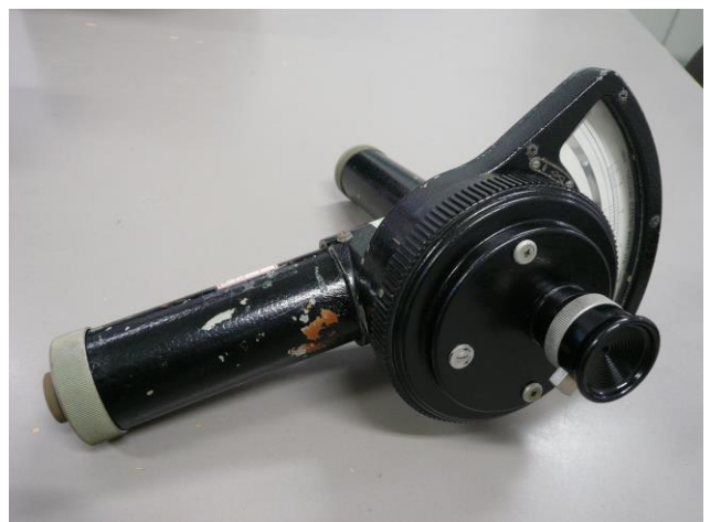
Radiation temperature meter using diminishing image of hot wire (corridor)
