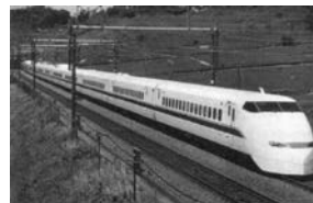
Model 300 (1992~) and Model 500 GTO + PWM control electric power regeneration brake
