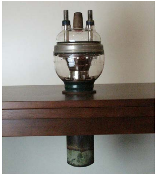
Water cooled triode for transmitter (8T72A))
