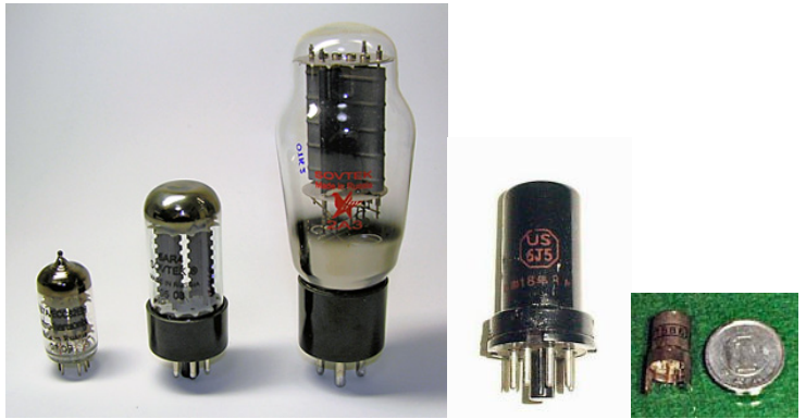
Diode Triode Triode MT tube, GT tube, ST tube, Metal tube, Nuvistor Fleming (1904) de Forest(1906) (Indirect heating)
