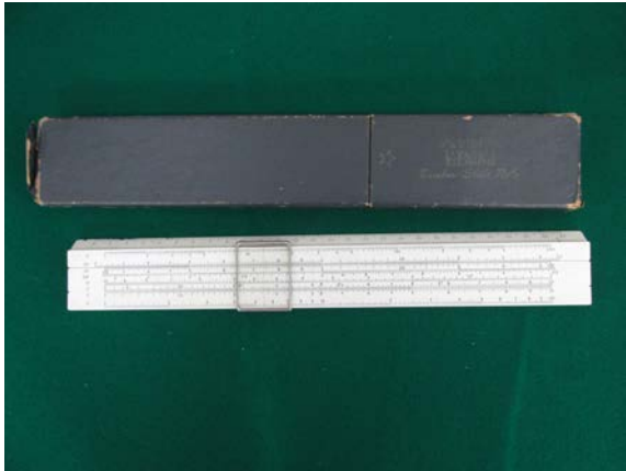
Bamboo Slide Rule[1] ( \log AB = \log A + \log B )
