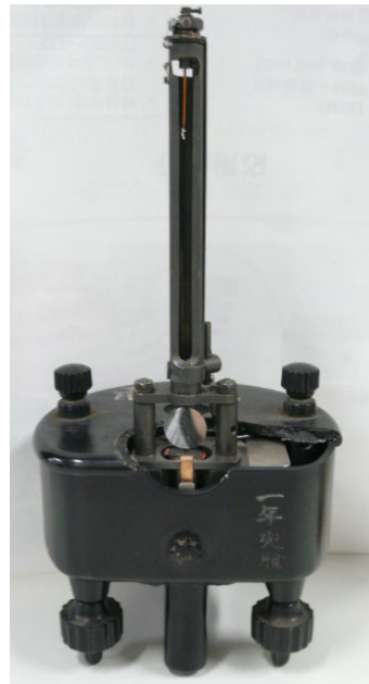
Potentiometer (measurement of electromotive force with zero current)
