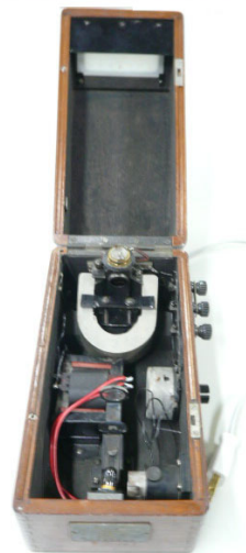
Optical galvanometer (2) (sensitivity 0.02 \mu A )
