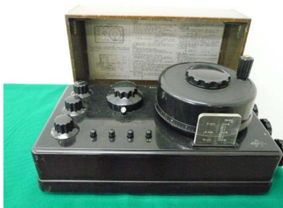
Potentiometer (measurement of electromotive force with zero current)
