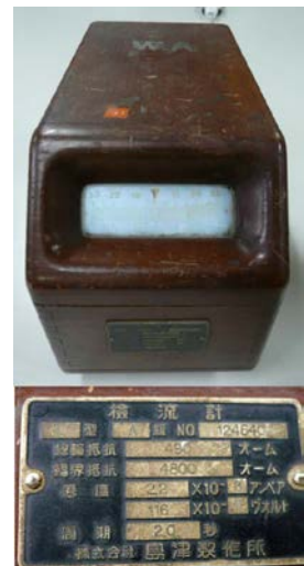
Optical galvanometer (2) (sensitivity 0.02 \mu A )
