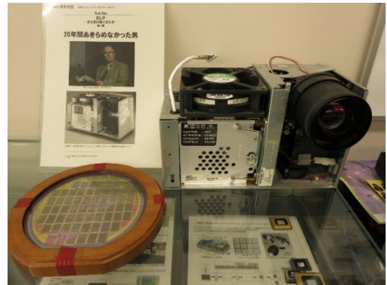
Mirror array (DMD) (TI) (Wafer, projector)
