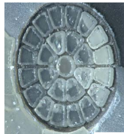
Forward-looking intravascular ultrasound imager and fabricated transducers, pulsar and amplifier ( \mu\text{SIC} ) (J. J. Chen et al. , Proc. of MEMS (2004))
