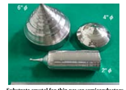
Substrate crystal for thin power semiconductors
