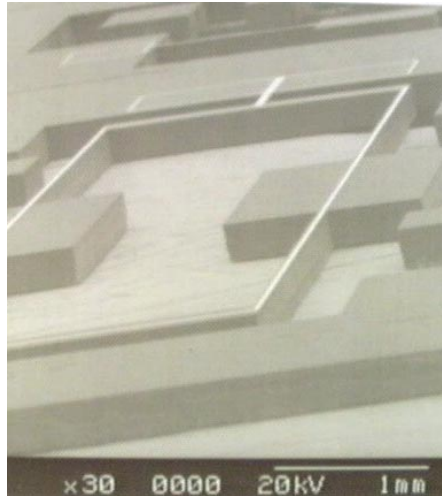
Deep RIE system and resonating gyro fabricated using it
