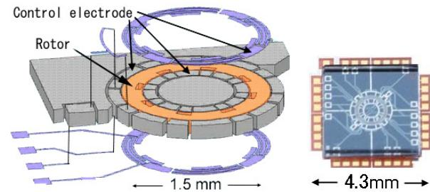
Yaw rate & acceleration sensor (Toyota motor Ltd.)
