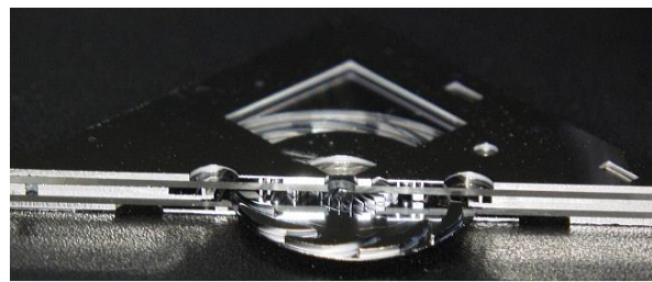
Si air-turbine with radial-inflow type journal bearing
