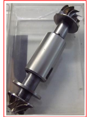
Gas turbine dynamo developed in IHI
