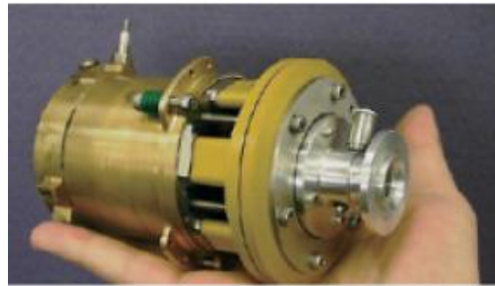
Gas turbine dynamo developed in IHI
