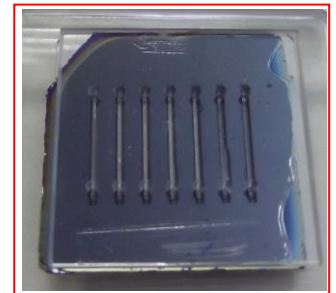
Absorptiometric analysis chip which hold chemical by surface tension (Tohoku Univ. – Friburg Univ. (Germany))
