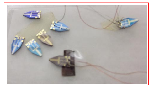
Electromagnetically driven AFM probe
