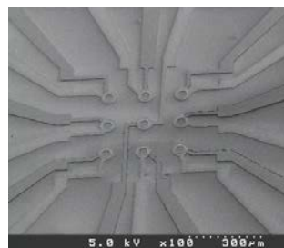
Carbon nanotube electron source with electrostatic lens
