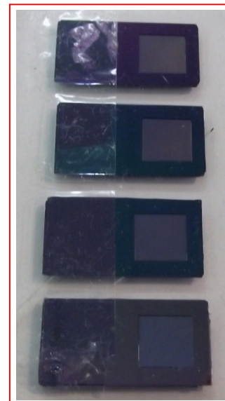
Thickness 2/3/5/7 \mu\text{m} from the top
