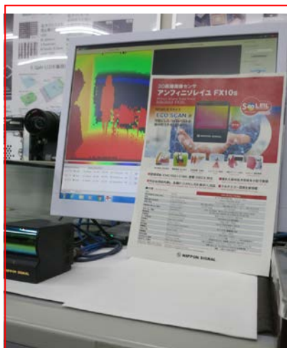
Ranging imager system “Eco scan” (Japan Signal) applied for platform door in railway station
