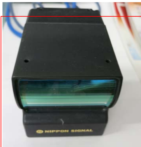
Ranging imager system “Eco scan” (Japan Signal) applied for platform door in railway station
