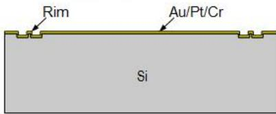
(b) Printing with Au paste and sintering at 200°C/2h in Ar-4%H<sub>2</sub>.
