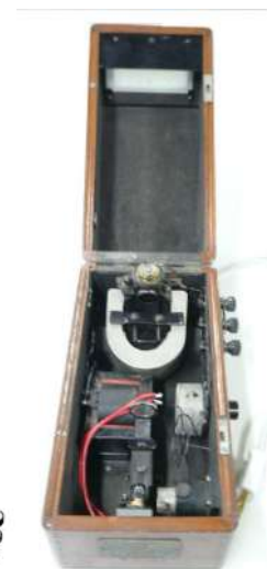
Optical galvanometer (2) (sensitivity 0.02 \mu\text{A} )
