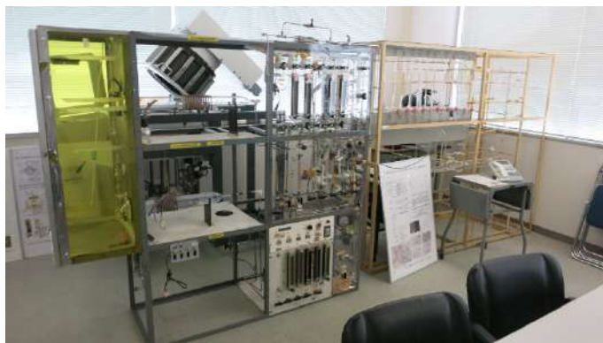
Glass pipe gas line for Si epitaxial growth system (right), atmospheric pressure CVD system (poly Si, Si 3 N 4 , SiO 2 ) (left)
