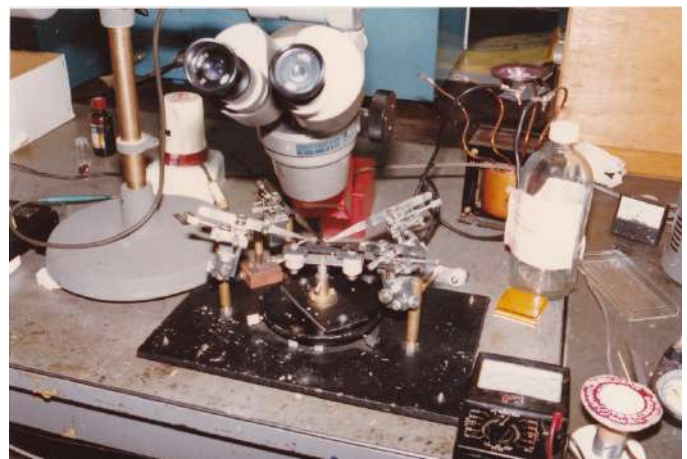
Micro soldering (and connection by conductive paste)
