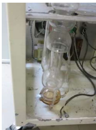
Oil diffusion pump (principle) and photograph of which K. Kumano made
