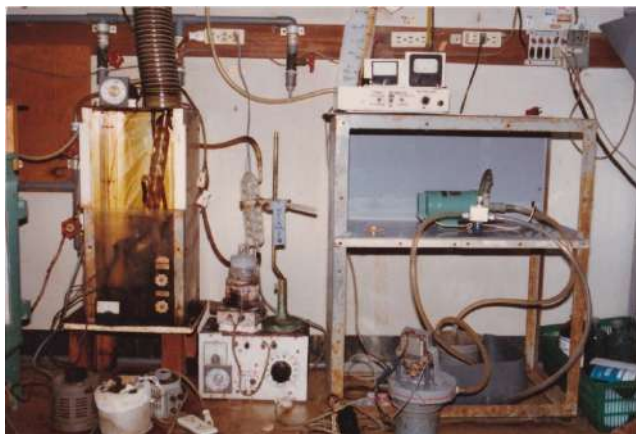
Si EPW etcher, SiN etcher in hot phosphoric acid, Electrochemical Si etcher DI water supply
