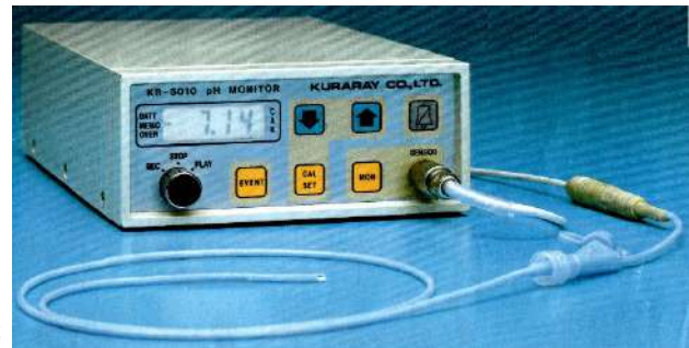
ISFET and reference electrode in 2.4mm diameter catheter
