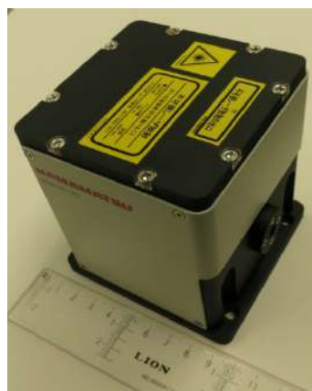
Quantum pulse cascade laser (Hamamatsu photonics) (commercialization based on Hands-on access fabrication facility)
