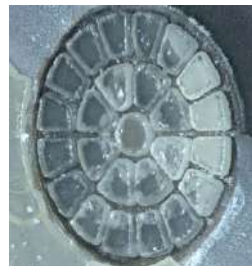
Forward-looking intravascular ultrasound imager and fabricated transducers, pulsar and amplifier (μSIC) (J. J. Chen et al. , Proc. of MEMS (2004))
