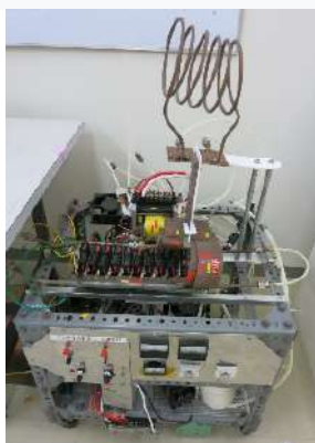
Oscillator for RF inductive heating using SIT (static induction transistor) (Token)(exhibited)
