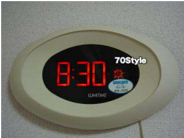
Mechanical discharge lamp display clock driven by AC motor (1970 Tamura) [1]
