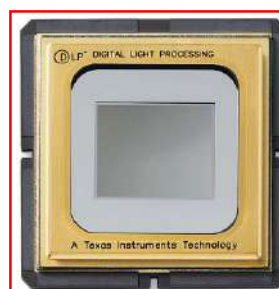
Mirror array for video projector DMD (Digital Micro mirror Device) (Texas Instruments (USA))
