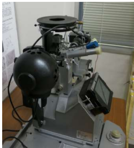
Phase difference microscope (Reichert MEF)
