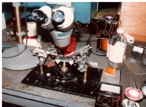
Micro soldering machine using cream solder (right exhibited)
