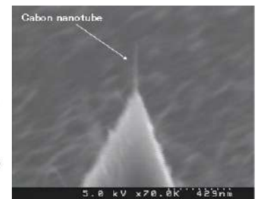
Hot filament CVD used for Carbon nanotube growth (or diamond film deposition).
