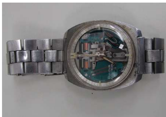
Tuning fork watch (1960 Bulova Accutron (Switzerland) [2]
