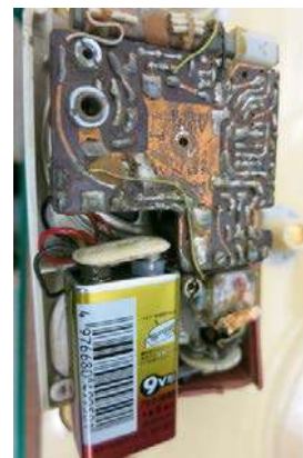
Transistor radio (Sony TRW-621)(1960) (Clock can be used as timer) [2]
