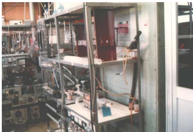
RF heating poly Si, SiO 2 CVD (top)
