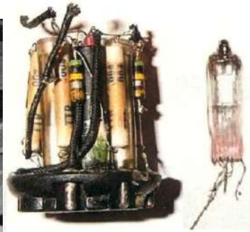
Electronics of VT fuse
