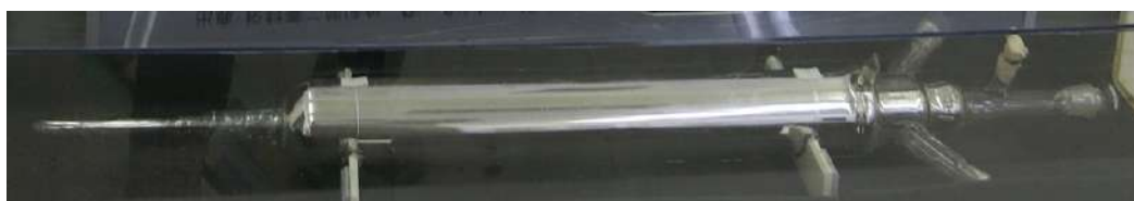
Double-duplex glass tube Helium cryostat Dewar Designed for long time measurement with minimal liquid Helium consumption
