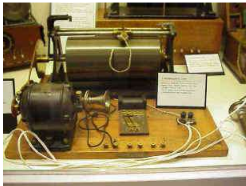
Magnetic wire recording by V. Poulsen (1898),
