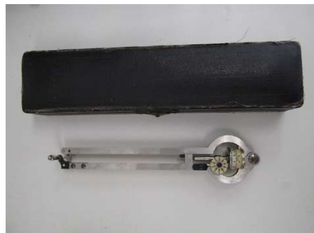
Planimeter (measurement of area)
