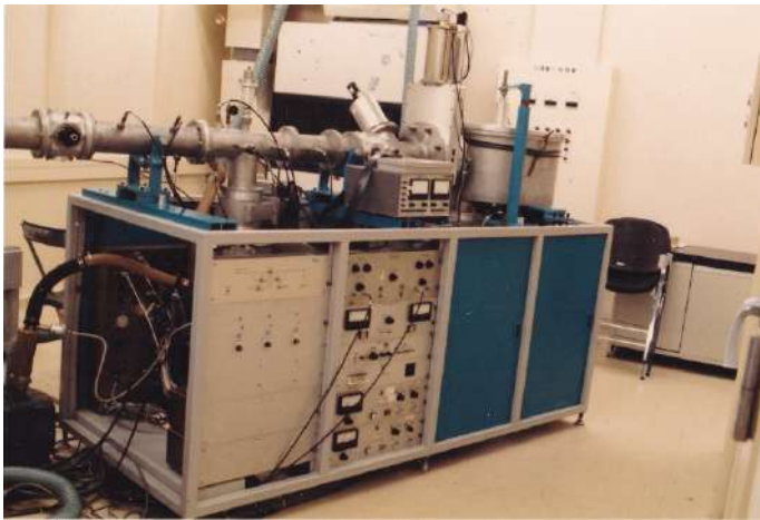
Ion implanter (Accelerator Inc, 200MP second hand)
