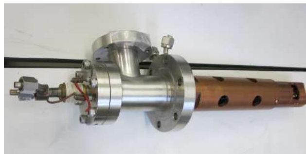
Xray source (exhibited) and its structure
