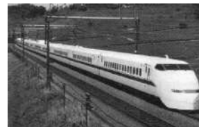
Model 300 (1992~) and Model 500 GTO + PWM control electric power regeneration brake Model 700 (1998~) IGBT Inverter
