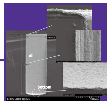
Si / SiO 2 W-CVD (via structure)
