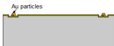
(c) Thermo-compression bonding at 200°C/30min under a pressure of 200MPa for the rim.
