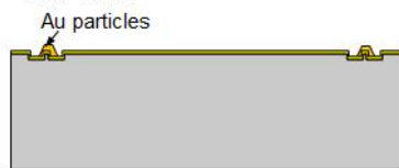
(c) Thermo-compression bonding at 200°C/30min under a pressure of 200MPa for the rim.
