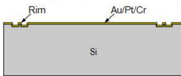
(b) Printing with Au paste and sintering at 200°C/2h in Ar-4%H 2 .
