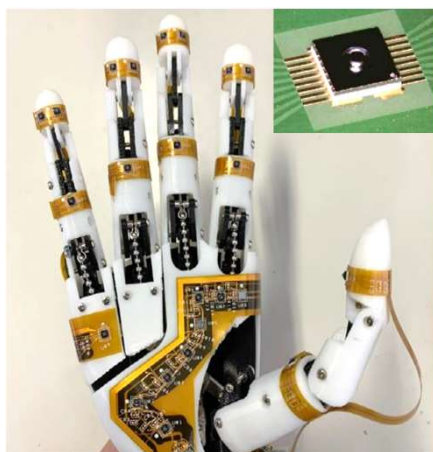
Fig. 2 Integrated tactile sensors on robot hand* *from Prof. Naoki Fukaya, TMCIT
